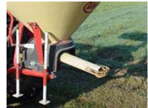
Figure 2. Spout on pendulum-action spreader.
